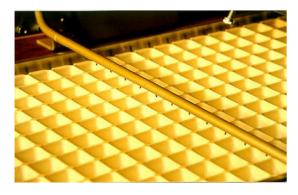
picked up by vacuum on the holes. The handle is then moved from the pickup position to the discharge position, just above the plug tray. A small hole in the handle is covered to release the seeds onto the surface of the compost. The tray is moved by hand to the next row, and the process repeated. The vacuum and vibration are adjustable for different sizes and weights of seed.
