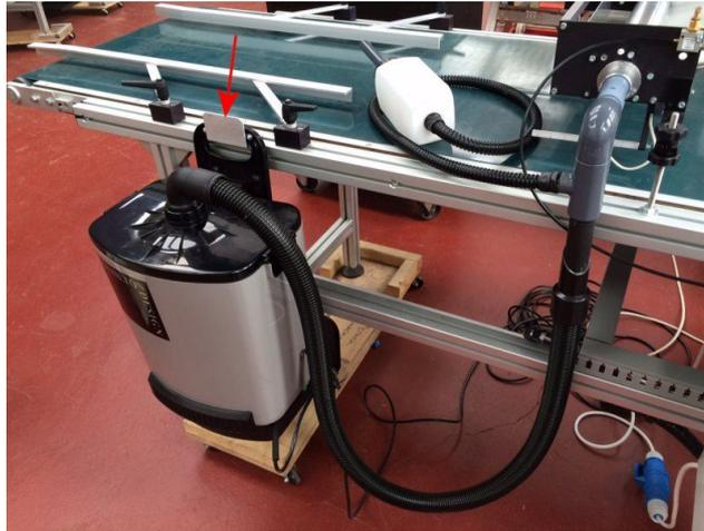
If you have the latest type drum seeder, disconnect the vacuum pump, and plug in the new vacuum. If you have the old drum seeder (green conveyor) remove the vacuum plug and connect to a separate electrical outlet with a suitable plug.
