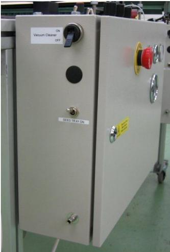
Turn on the seeder power switch on the top of the main control box. Switch the seed tray switch on the end of the control box to the down position. The tray will run until the switch is lifted, or the main power is turned off. Avoid running the tray for long periods without sowing, to preserve the life of the anti-wear impregnated fabric material.
